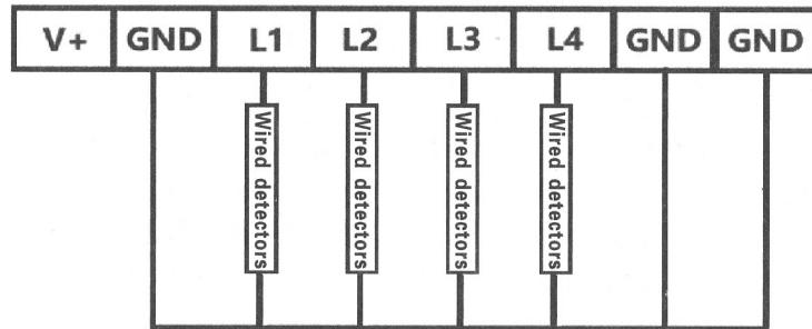
**Note :** v+ provides a single power output, which can output 9V DC power to provide wired accessories when an external power supply is applied. Please refrain from supplying power to high power loads.
